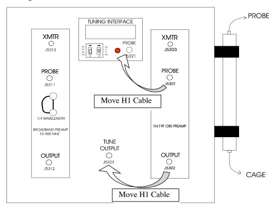
9. When completed, change the CHAN channel back to 0 by pressing the - key once. The TUNING INTERFACE readout should blank, and the red light should start blinking.
